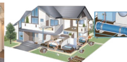
Potable water storage system Fresh drinking water stored in the water pipes underfloor, and easily withdrawn in the event of water outage
